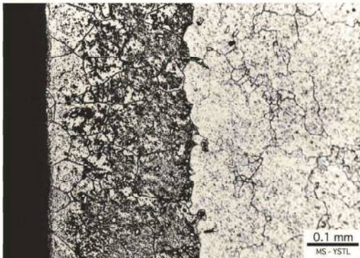
Standard piece No.54 Decarburized structure
