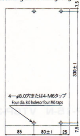
取付穴加工図 Mounting hole drilling diagram
