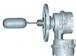
FB-9000 -Bellows type -Pressure: 0.2 MPa (option: 2 MPa) -Temperature range: -19 to 150°C -Material: Stainless steel -Switch: Microswitch, air microswitch
