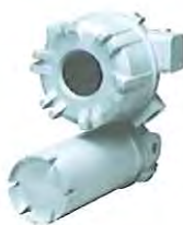
FDC-1000 -Field device controller -Contact output: Max. 8 points -4 to 20 mA DC: Max. 2 points -Contact input: Max. 8 points -Indication: Contact input status, contact output status, 4 to 20 mA DC status
