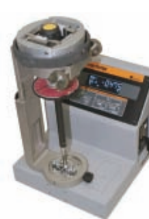
Calibration figure for torque screwdriver RTD left and FTD right with TDT3-G
