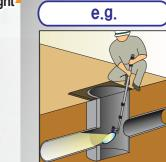
Useful for checking inside of the pipe from manhole, etc.
