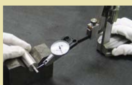
Determination of channel width
