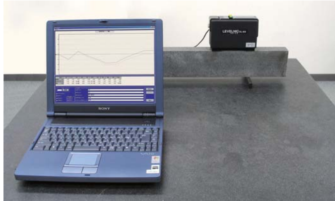
■ Straightness measurement while connected to PC
