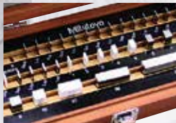
CERA/Steel Combination Gage Block Sets
