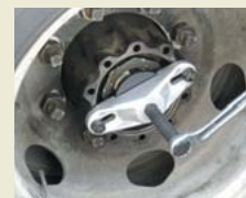
*An off-set wrench (with 27mm width across flat) or a socket with a drive tool (sold separately) is required for operation.
