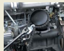
*A 1/2"sq spinner handle or an off-set wrench (with 24mm width across flat) (sold separately) is required for operation.
