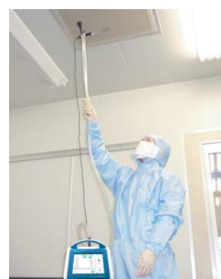
Climomaster™ probe for environmental measurements
