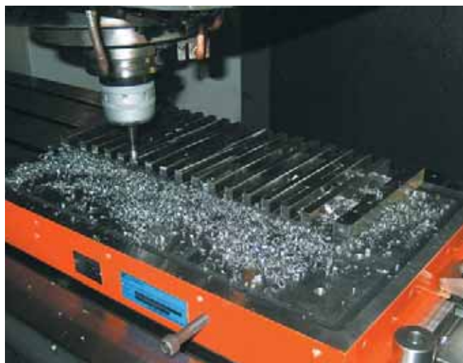
An example of machining by use of straightening block
