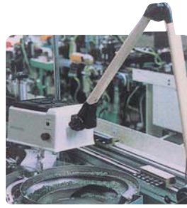
Example of neutralization of electronic parts in a parts feeder.
