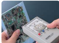
Ionizing air blower's ion balance adjustment
