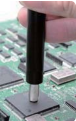
DT-510 + DT-510C usage example (IC surface temp., solid surface temp.)
