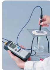
DT-510 + DT-510C usage example (IC surface temp., solid surface temp.)
