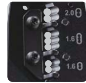
Outer jacket stripping hole
