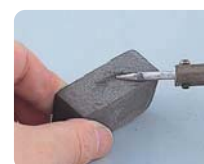
Soldering iron tip cleaning (The soldering iron tip should be cooled before cleaning it.)
