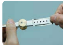
The grasping pressure is adjusted by sliding the spring
