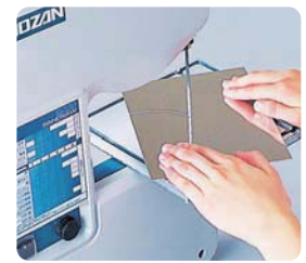
Cutting an aluminum sheet along a curved line
