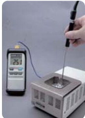
DT-510 + DT-510A usage example (solder bath temperature, liquid temperature)
