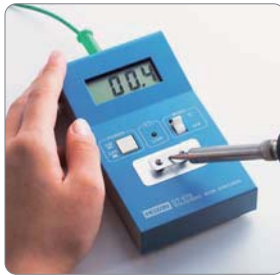
Example of ground resistance measurement (See below for details of the measurement method)
