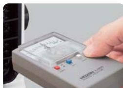
Ionizing air blower's ion balance adjustment
