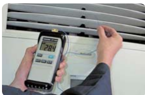
DT-510 + DT-510B usage example (air-conditioner outlet temperature)
