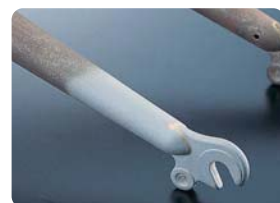
Surface preparation before painting (#120 abrasive used)
