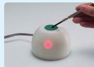
Demagnetizing a screwdriver.
