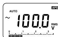
Measuring 100 V using the 300 V range
