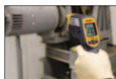
Locations that cannot be touched due to moving parts
