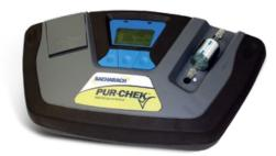
Pur • Chek™ is smarter and faster than any refrigerant identifier used in the industry today. Its compact size and ergonomic design makes testing easy and it utilizes non-dispersive infrared (NDIR) technology to determine the weight concentrations of R-12, R-1134a, R-22, hydrocarbons and air. It also features 'Blend-Chek' analytical software which quickly and accurately indicates the presence of R-410a blend refrigerant.
